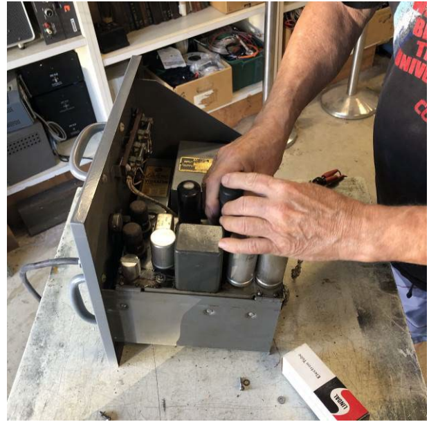
Bill tested the vacuum tubes inside of the amps and supplied working tubes for those missing. Now both Megaphones and amps are tested good.
