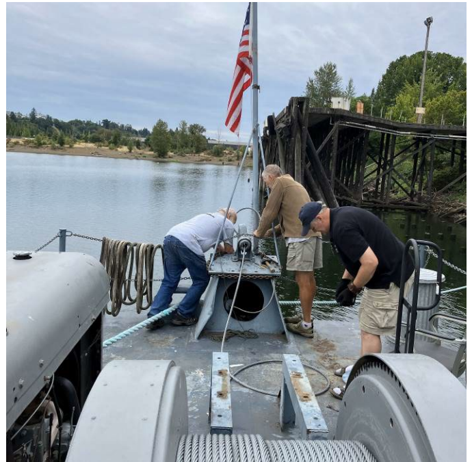
The crew loading 1000 feet of wire cable onto the winch drum and connecting to anchor.
