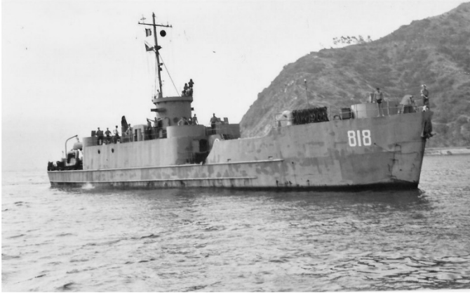
The LCI(L) 818 was beached on Iheya Island when the war ended. This photo shows the ship after the war, stripped of most guns and serving as LSI(L) 818 training ship.
