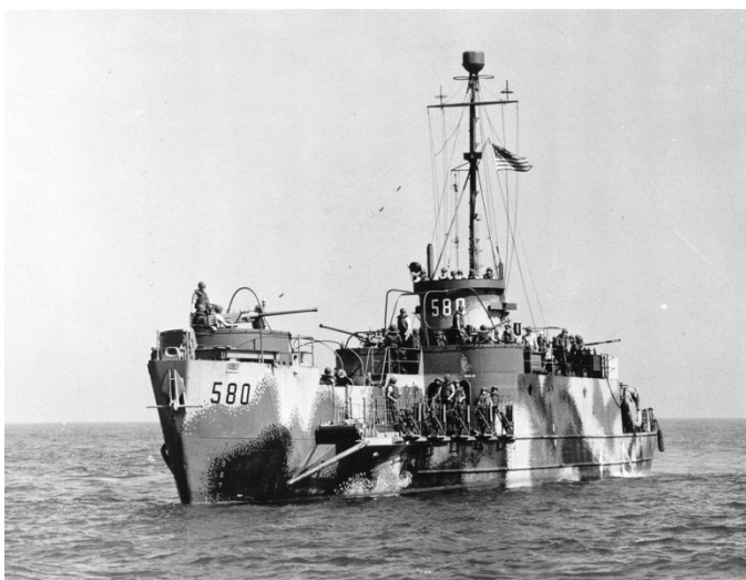
LCI(G) 580 with all battle stations manned. The five portside rocket launchers are visible.
