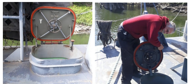
New gaskets for all the hatches
