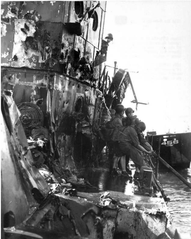
LCI(L) 339 at Lae New Guinea settled on the bottom showing the damage from a Japanese Bomb
