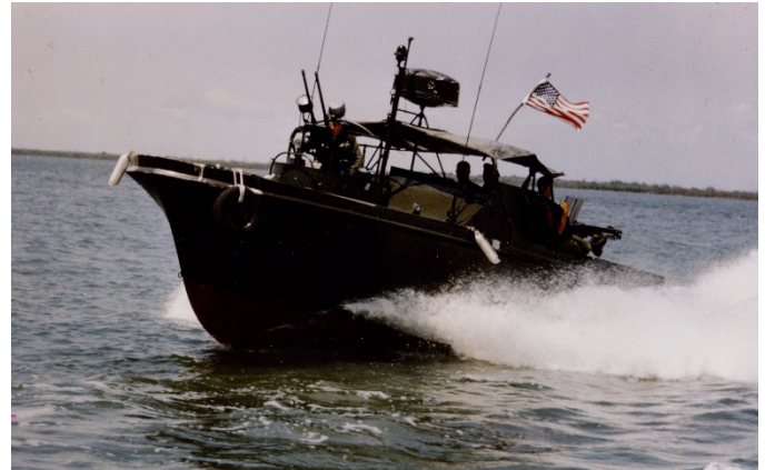
The 32-foot PBR could reach speeds of 28.5 knots with two 180hp Detroit diesel engines.
