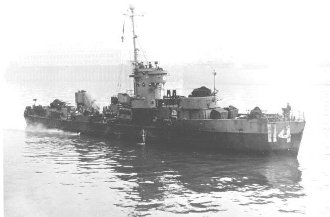
LCS(L) 114 was a rocket-firing gun boat. She was built on the same hull as an LCI.
