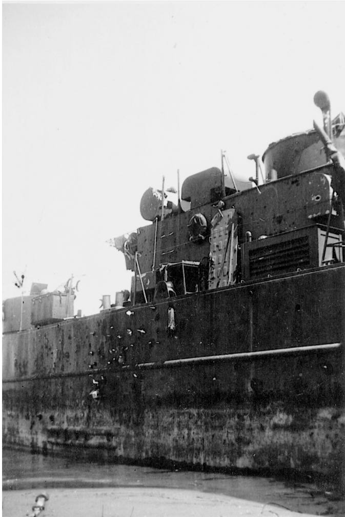
LCI(G) 23 bomb damage. Note the wooden plugs sticking out of the hull.
